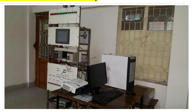
This lab is located at 1<sup>st</sup> floor of Academic Building-2. Trainers are introduced to the principles and methods of automatic level control loop with advanced programmable instruments.
