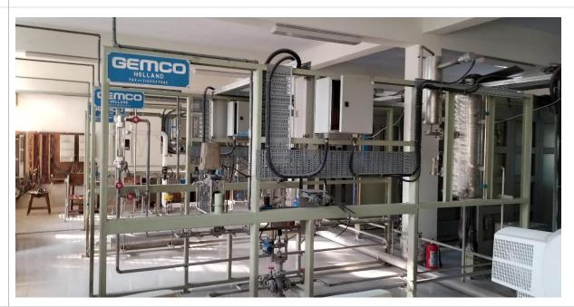
This lab is located at Ground floor of Academic Building-2. DCS Pilot plant is a fully computerized system incorporating practical facilities on computerized process control and automatic startup shutdown logic interlock widely used in industries.
