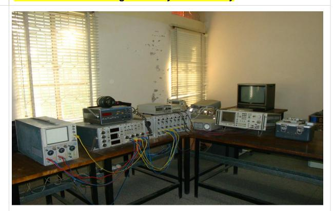
This lab is located at 1<sup>st</sup> floor of Academic Building-2. Facilities of this lab include highly sophisticated vibration monitoring and analysis equipment for on-line troubleshooting of rotating machines.
