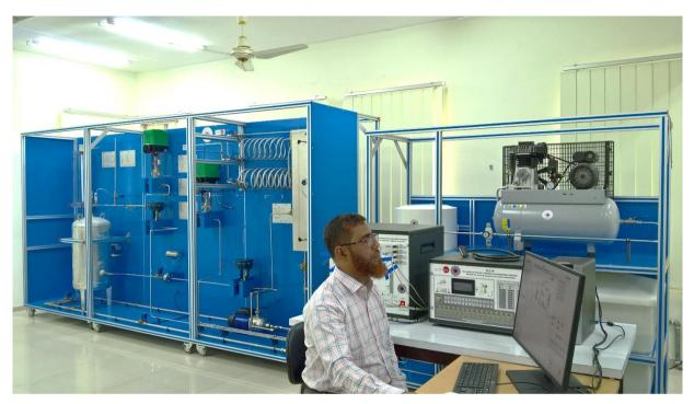
Fig: Process Control Plant with SCADA & PID control
