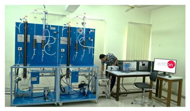
Fig: Double Effect Rising Film Evaporator with SCADA and PID Control
