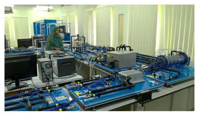
Fig: Heat Exchange Training System with SCADA and PID Control
