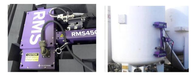
Fig: RMS2 450 for Tank & Pipeline corrosion testing and profiling
